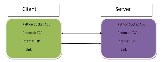
TCP (Transmission Control Protocol) is a standard that defines how to establish and maintain a network conversation through which application programs can exchange data. TCP works with the Internet Protocol (IP), which defines how computers send packets of data to each other. Together, TCP and IP are the basic rules defining the Internet. The Internet Engineering Task Force (IETF) defines TCP in the Request for Comment (RFC) standards document number 793.
