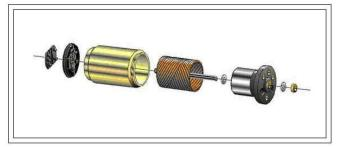
The coreless design also allows manufacturers to build smaller motors; meanwhile,due to the lack of iron in their rotors, coreless motors are somewhat prone to overheating. As a result, this design is generally used just in small, low-power motors. Beamers will most often see coreless DC motors in the form of pager motors.
