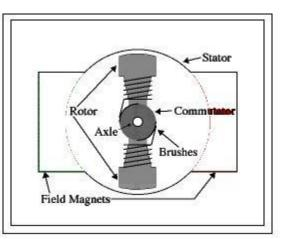
magnetic field. As you are well aware of from playing with magnets as a kid, opposite (North and South) polarities attract, while like polarities (North and North, South and South) repel. The internal configuration of a DC motor is designed to harness the magnetic interaction between a current-carrying conductor and an external magnetic field to generate rotational motion.
