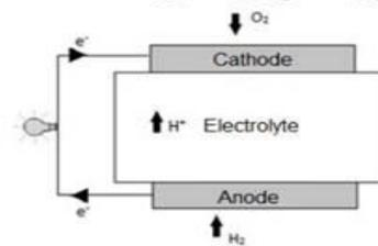
Fig2. Basic Configuration of Fuel Cell
