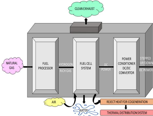
Fig3. Fuel Cell Cogeneration System
