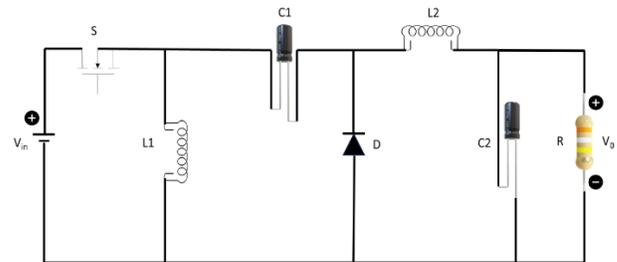
Fig5. ZETA Converter [DC-DC Converter]
