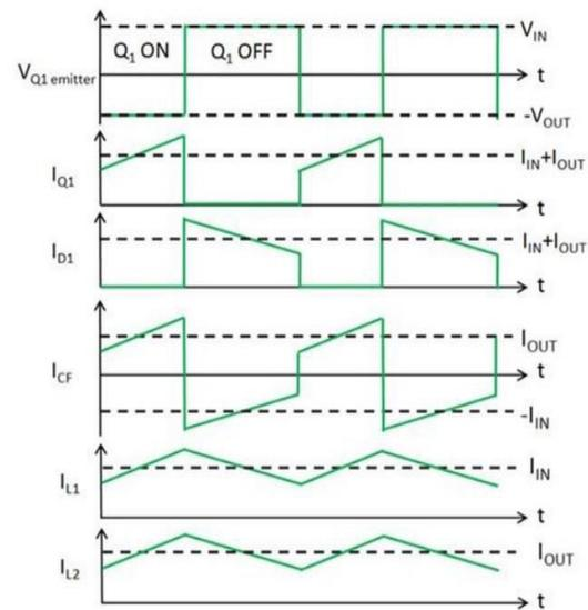
Fig6. Waveforms of elements in the ZETA Converter circuit [6]
