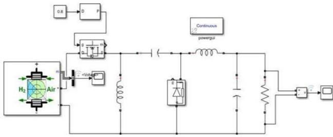
Simulation model of ZETA converter with Fuel cell
