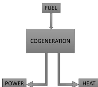
Fig1. Principle Functioning of Cogeneration
