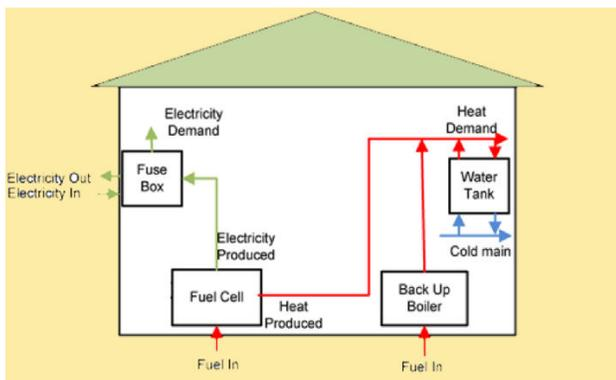
Fig4. Domestic Usage of Fuel Cell Cogeneration System
