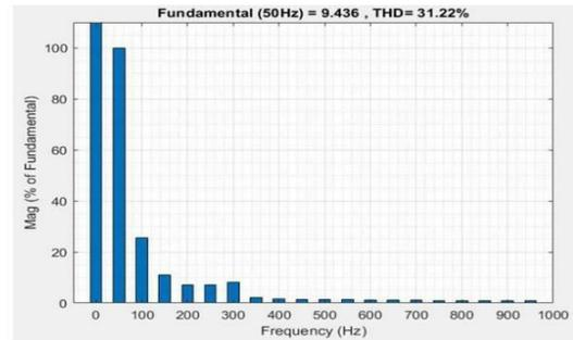
Voltage THD analysis waveform of ZETA converter
