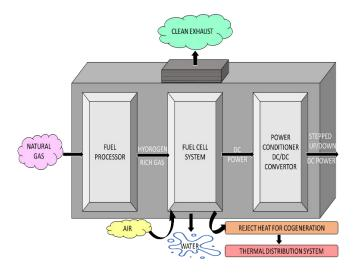
Fig3. Fuel Cell Cogeneration System
