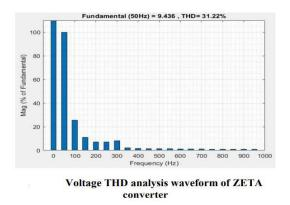
The low Total Harmonic Distortion (THD) value of ZETA converter implies that there is room for improving the efficiency of the converter, when compared to converters of high THD values.
