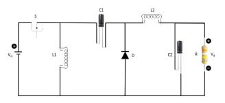
Fig5. ZETA Converter [DC-DC Converter]
