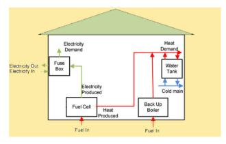
Fig4. Domestic Usage of Fuel Cell Cogeneration System
