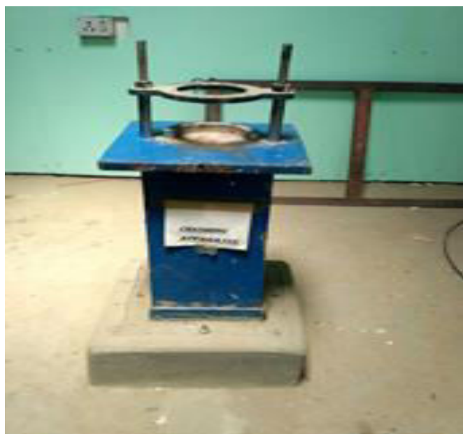
Fig. 3 Crushing Strength Apparatus
