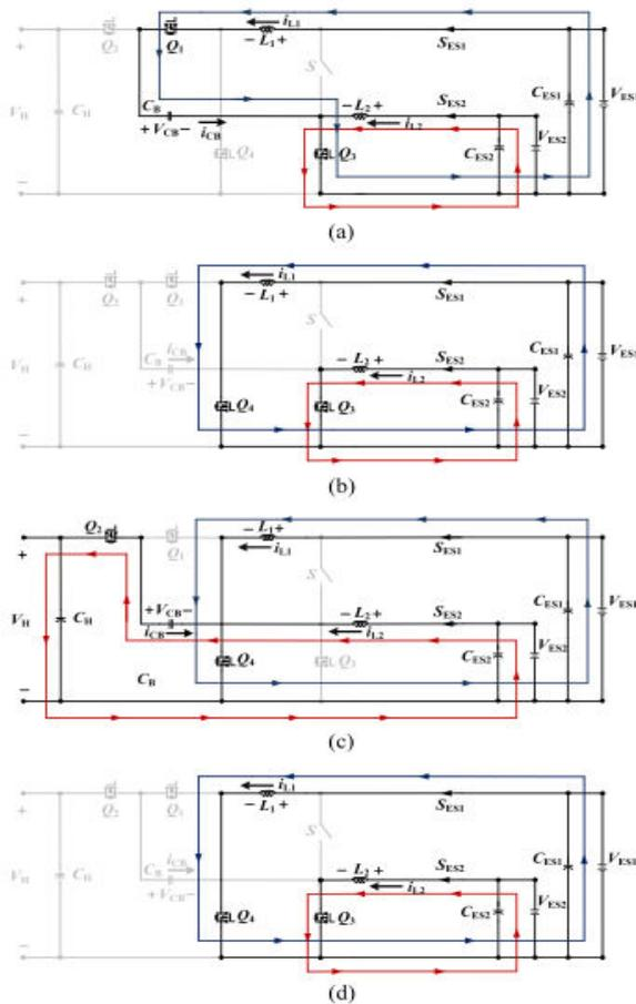
Fig. 2.2 Circuit states of the proposed BDC for the low-voltage dual source-powering mode (a) state 1 (b) state 2 (c) state 3 (4) state 4
