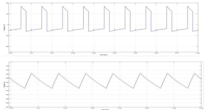
Fig:4(c). Voltage across the inductor (L2)
