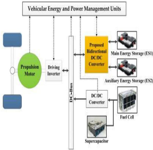
Fig.1. Diagram of a fuel cell/ hybrid electric vehicle system
