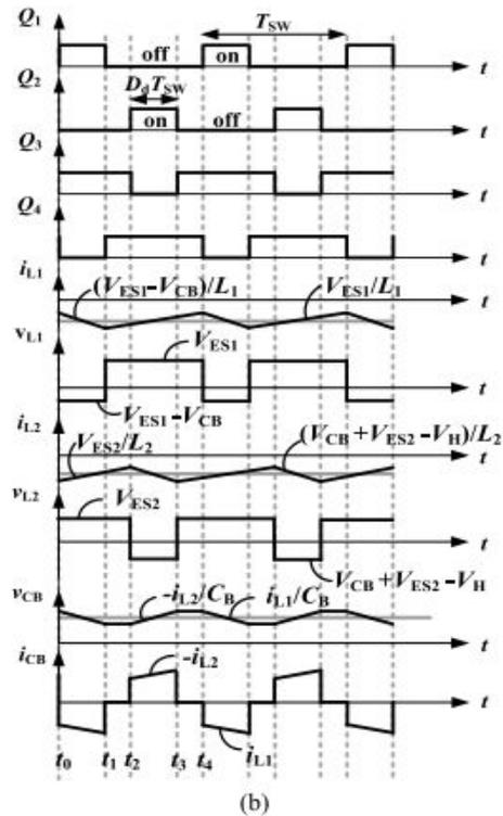
Fig.2.3 High-voltage dc-bus energy regenerating mode of the proposed BDC:
