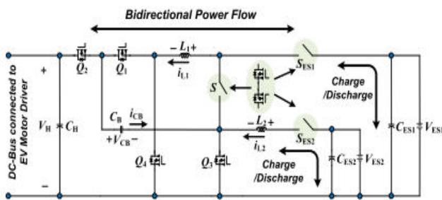
Fig. 2 Bidirectional dc converter topology with dual battery energy storage.
