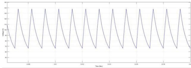
Fig.4 (d). voltage across the inductor (L1 and L2) and capacitor Voltage ( $V_{CB}$ )
