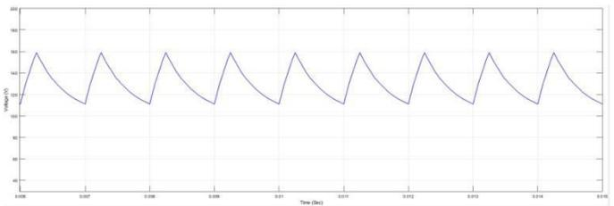
Fig:4(b) voltage across the inductor (L2) and capacitor voltage( $V_{CB}$ )
