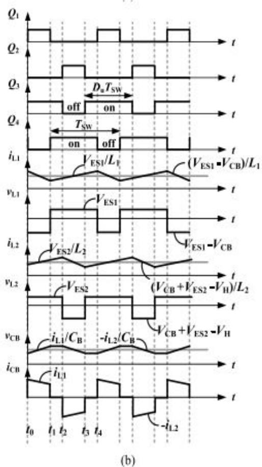
Fig. 2.1 Low-voltage dual-source –powering mode of the proposed BDC: (a) circuit schematic and (b) steady state waveform
