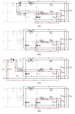
Fig. 2.2 Circuit states of the proposed BDC for the low-voltage dual source-powering mode (a) state 1 (b) state 2 (c) state 3 (4) state 4
