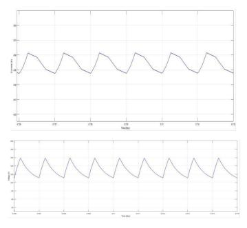
Fig:4(b) voltage across the inductor (L2) and capacitor voltage( $V_{CB}$ )
