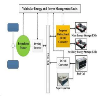
Fig.1. Diagram of a fuel cell/ hybrid electric vehicle system
