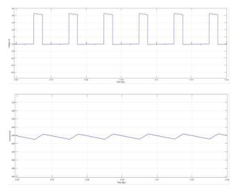
The response of source and load current waveforms produced by the above simulink model is shown in below fig.4(b).
