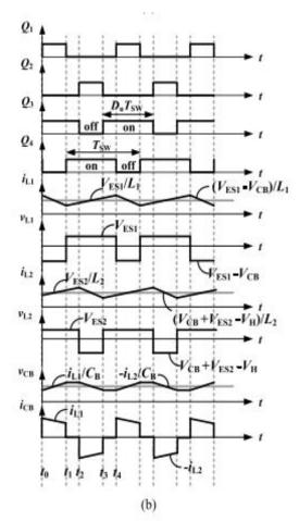
Fig. 2.1 Low-voltage dual-source –powering mode of the proposed BDC: (a) circuit schematic and (b) steady state waveform
