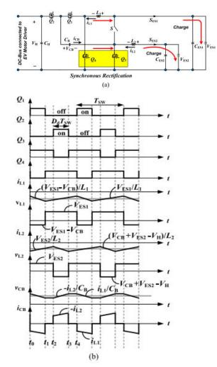
Fig.2.3 High-voltage dc-bus energy regenerating mode of the proposed BDC:
