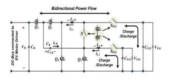
Fig. 2 Bidirectional dc converter topology with dual battery energy storage.
