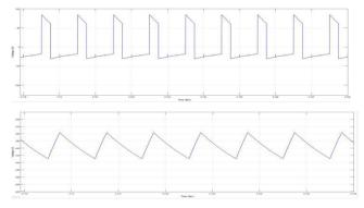
Fig:4(c). Voltage across the inductor (L2)
