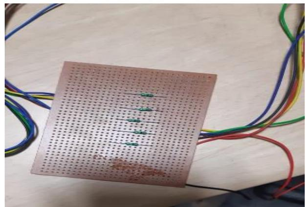
**Fig 1.6 voltage divider circuit**
