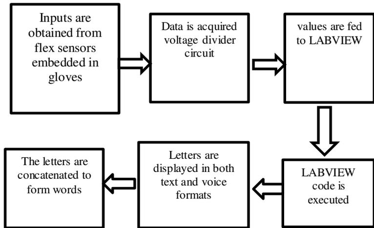
Fig 1.2 Block diagram of proposed system
