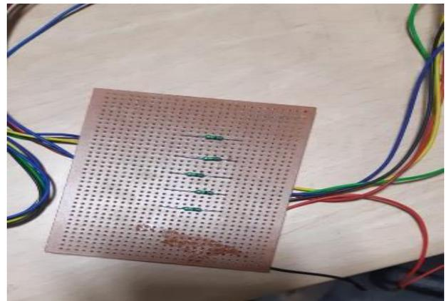
**Fig 1.6 voltage divider circuit**
