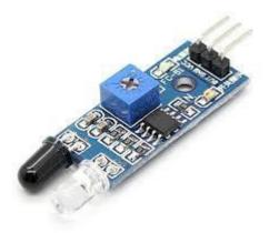
An infrared sensor is an electronic instrument that is used to sense certain characteristics of its surroundings. It does this by either emitting or detecting infrared radiation. Infrared sensors are also capable of measuring the heat being emitted by an object and detecting motion.
