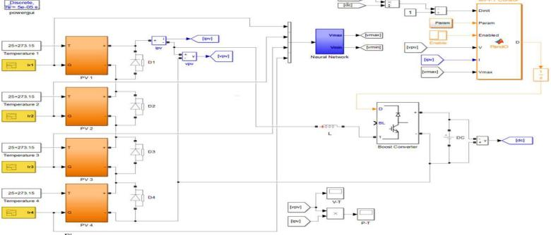
Fig. MATLAB/Simulink model of the proposed system.
