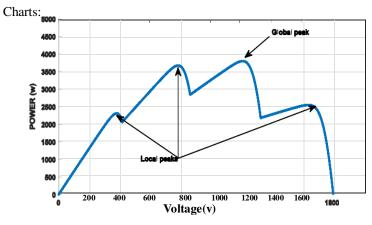
fig. 4. Photovoltaic array characteristics under the partial shading
