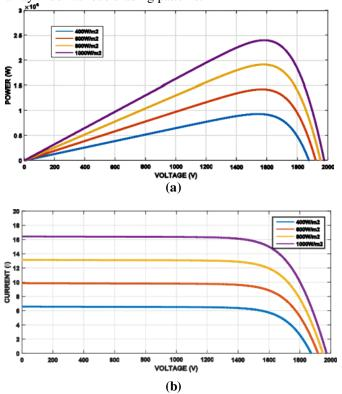
Fig. Photovoltaic array characteristics:-(a) Power-voltage curve. (b) Power-current curve.
