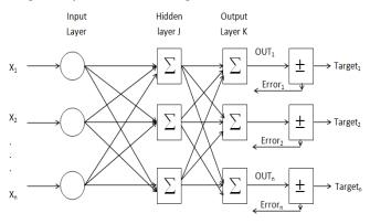
Fig. 3. The Back-Propagation ANN Structure
