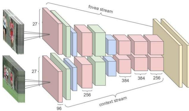
Figure 2: Multi-resolution CNN architecture. Input frames are fed into two separate streams of processing: a *context stream* that models low-resolution image and a *fovea stream* that processes high-resolution center crop. Both streams consist of alternating convolution (red), normalization (green) and pooling (blue) layers. Both streams converge to two fully connected layers (yellow).
