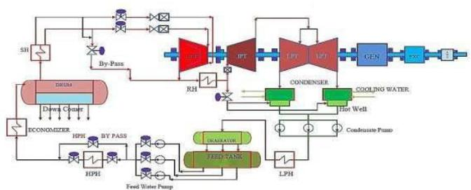
Fig. 1: Process flow diagram of the power plant
