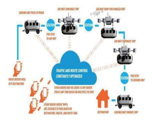
The air unit and ground unit are autonomously controlled, in constant communication with central traffic controlling and route managing system. A human pilot/driver can be on board to act as an emergency safety backup, but would not be able to fly the vehicle in normal operation[1].
