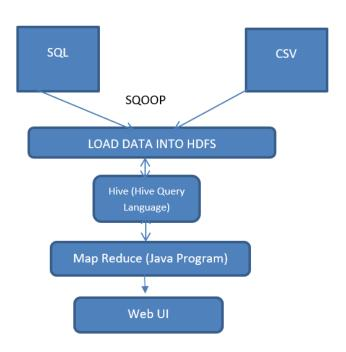
This architecture explains the interaction or stream of the task. First we ought to imports document into HDFS to preparing that enormous information in Hadoop open source system. Furthermore, we can handle that information with the assistance of three tools in particular hive and at long last we get yield what we need result from the dataset, what we have in this undertaking.
