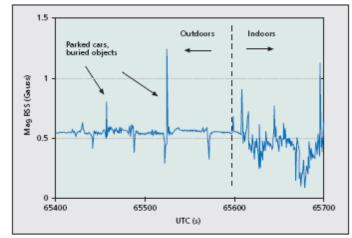
Figure 5. Sample measured magnetic RSS, outdoors to indoors.
