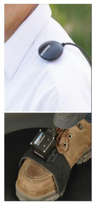
Figure 1:The IMU and embedded magnetometer
