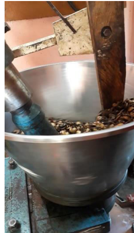
Figure 2 Extraction of oil by cold press method
