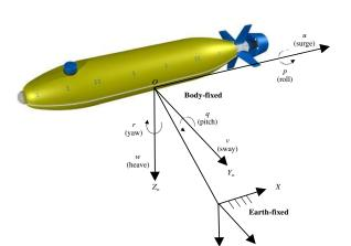
Figure-2. Body-fixed and earth-fixed reference frames
