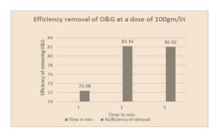
**6.2** Graph No. 2- Graph of oil and grease removal efficiency for sugar cane bagasse dose of 100gm/lit
