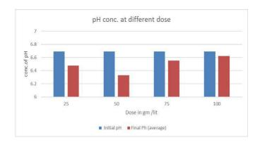
Following graph shows effect of sugarcane bagasse on pH of waste water
