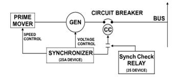
**Figure.10** Automatic Synchronizing
