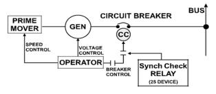
Figure.9 Manual synchronizing with synch check relay
