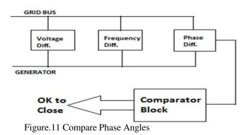
The synchronizer senses frequency, phase and bus voltage of both generator and therefore the grid
