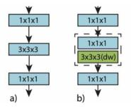
Fig-2: (a) A standard ResNet bottleneck block. (b) An interaction preserved bottleneck block.
