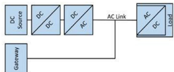
Figure 3. Block diagram of AC nanogrid [13].
