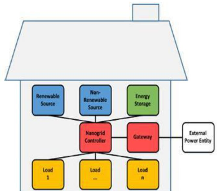
Figure 1. Block diagram of Nanogrid system [13].
