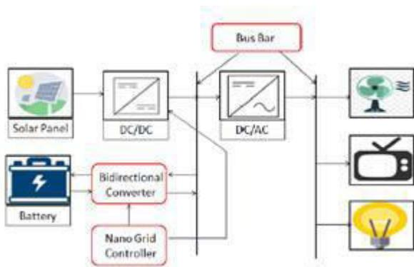
Figure 4. Block diagram of standalone PV based Nanogrid System [1].
