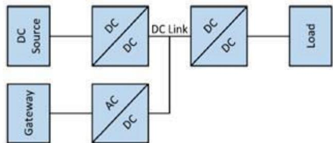
Figure 2. Block diagram of DC nanogrid [13].
