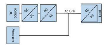
Figure 3. Block diagram of AC nanogrid [13]. The arrangement that consists of AC/DC and DC/AC converters is also referred to as frequency converter, since it
