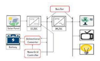
Figure 4. Block diagram of standalone PV based Nanogrid System [1].
