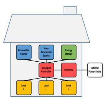
Figure 1. Block diagram of Nanogrid system [13].
