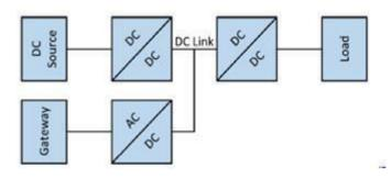
Figure 2. Block diagram of DC nanogrid [13].
