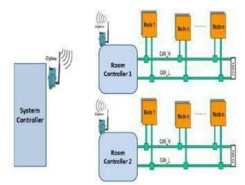
Figure 5. LVDC multilayer communication network [6].
