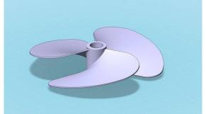
longitudinal axis, giving the propeller an overall cup-shaped appearance. This design preserves thrust efficiency while reducing cavitation's, and thus makes for a quiet, stealthy design.
