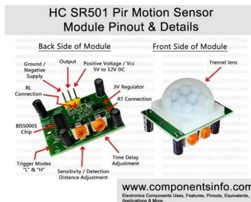
Fig – 4: Passive Infrared Sensor
