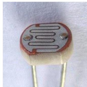
Fig – 3: Light Dependent Resistor Sensor
