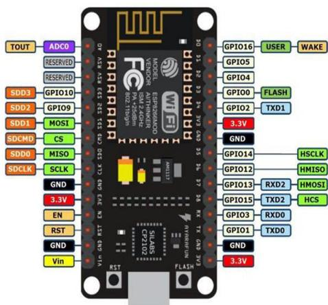
Fig – 5: Node MCU Controller (ESP8266)
