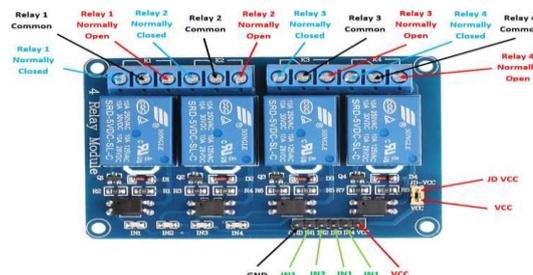
Fig – 7: 4 – Channel Relay Module
