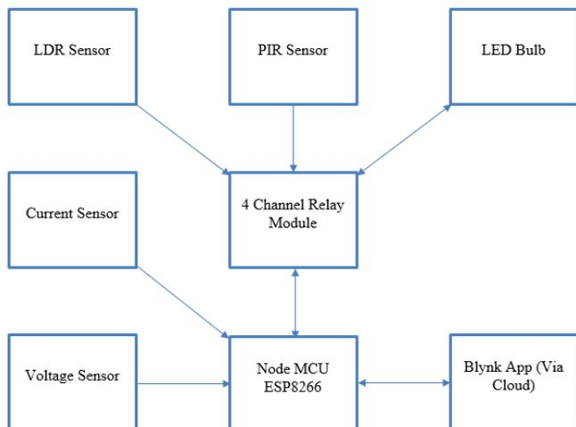
Fig – 9: Block Diagram of Smart Street Light System
