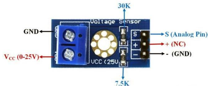
Fig – 1: Voltage Sensor
