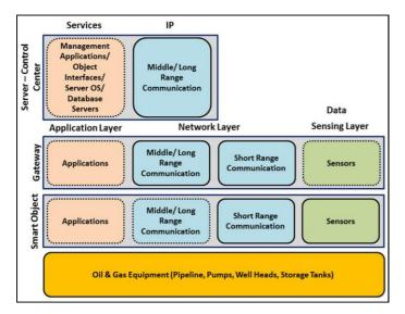
Figure 1. Proposed IoT based Architecture for Oil and Gas Industries
