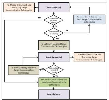
Figure12art representing how the proposed system will reliably, efficiently and accurately communicates the sensed information to the control center.
