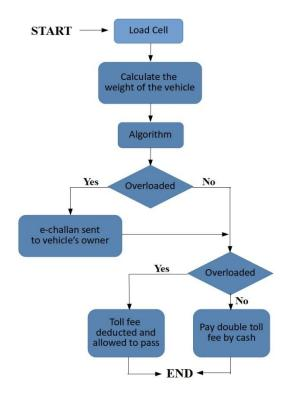
Fig - 4: Calculating the vehicle weight Flow Chart
