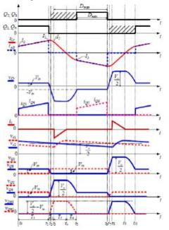
Fig:3.9 Operating waveforms of the proposed converter
