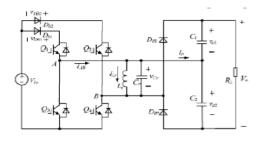
Fig:2.1 Proposed step up resonant converter
