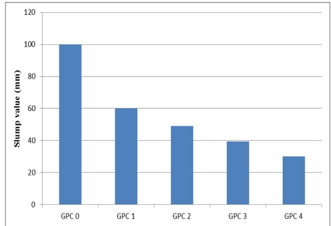
**Chart-8:-** Workability graph for different mix of geopolymer concrete
