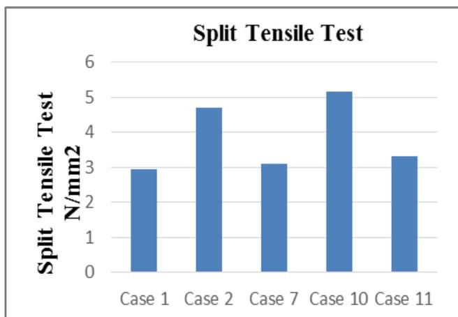
**Chart-11:-** Comparison of Split tensile strength test
