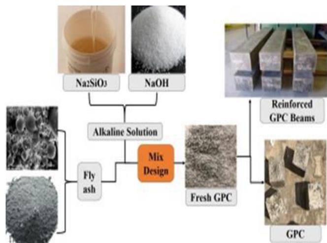
**Fig.1** Flow chart of Geopolymer concrete
