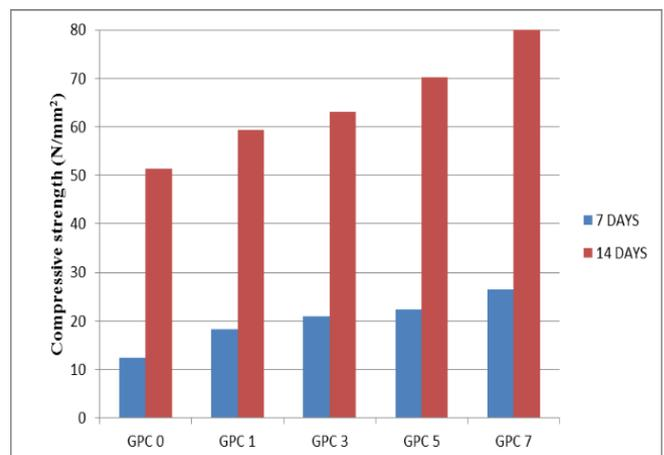
**Chart-9:-** Effect of inclusion of hooked steel fibers on compressive strength
