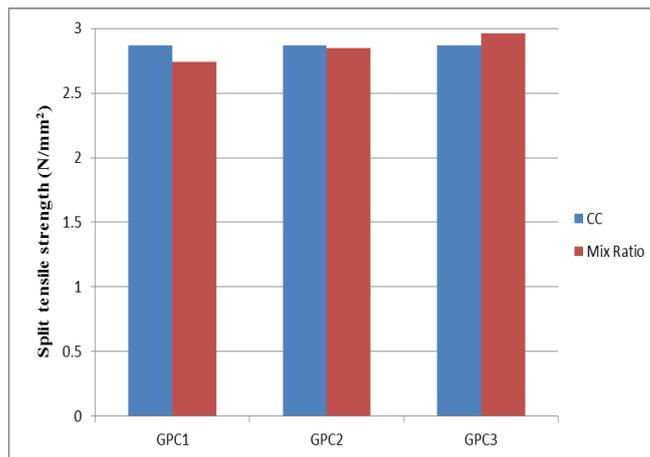
**Chart-6:-** Split Tensile Test of specimens at the age of 28 days
