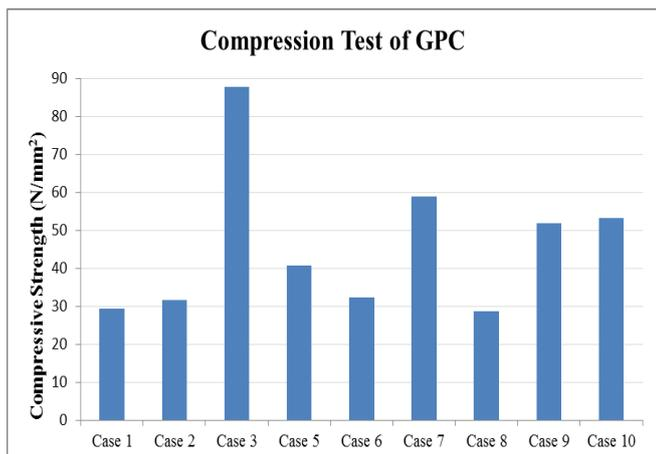
**Chart 10:-** Comparison of Compressive strength test
