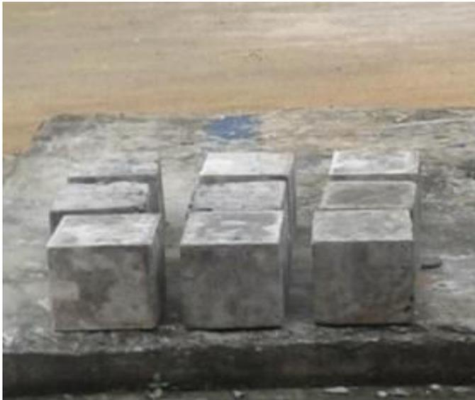
Fig. 3 Curing at ambient temperature
