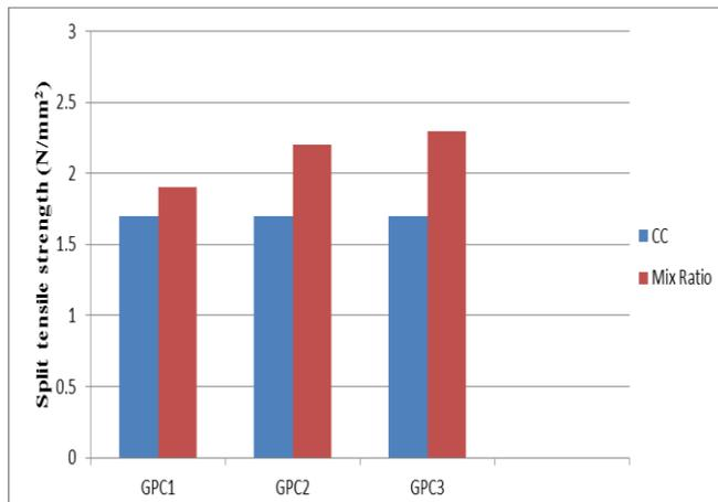
**Chart-4:-** Split Tensile Test of specimens at the age of 7 days
