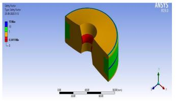
Fig 5. Half sectional 90mm diameter die with factory of safety value range 2.
