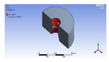
Fig 3. The Force 15000N applied to 90mm Die the at upward position
