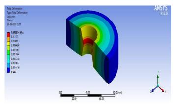
Fig 2. Total Deformation for 90mm Diameter Die.
