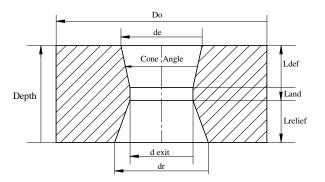
Fig 1: Conventional Die with all parameters
