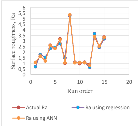
Fig 7.7 Comparison of actual Ra, Ra predicted by regression model and Ra predicted using ANN
