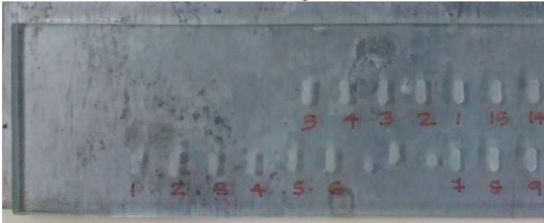
Fig 7.4 Fluidic channels machined using G-ECDM
