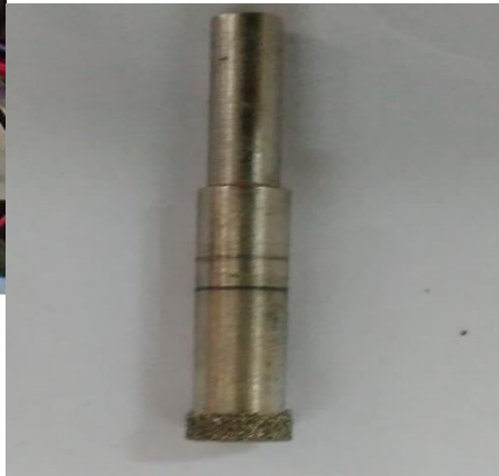
Fig. 7.3 G-ECDM tools (a) diamond coated engraving tool (b) core drill bit
