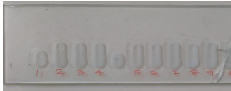
Fig. 7.10 G-ECDM using diamond core drill bit
