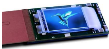
Fig. 4. Wearable display using microLED
