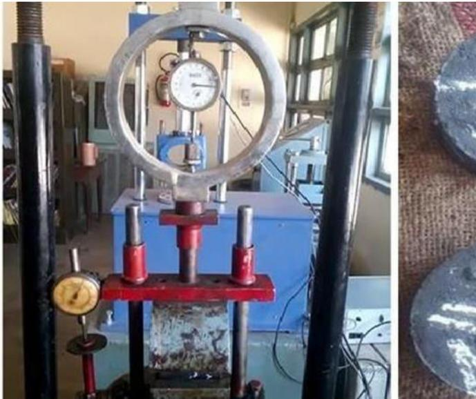
Fig -5: Marshall Machine Test
