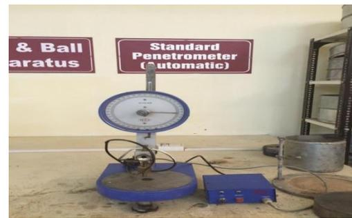
Fig -3: Penetration Test Apparatus
