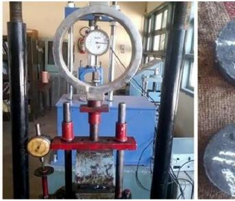
Fig -5: Marshall Machine Test
