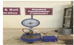
Fig -3: Penetration Test Apparatus
