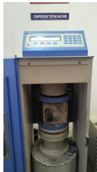
Fig -5: Compression Testing Machine
