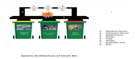
It is illustrated as, when the waste item, is kept on the plate, the respective sensors identifies whether the waste is wet or dry, and if it is dry, it further slides over to its respective bin area of metallic dry waste or non-metallic dry waste accordingly. The wet waste is collected and left out. From which we could identify further as plastic wastes that falls into the bin. And it is collected for further usage after segregation is done.
