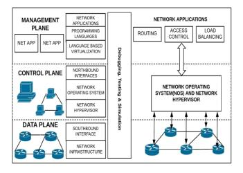
**Fig -2:** Software-Defined Networks in (a) planes, (b) layers, and (c) system design architecture.
