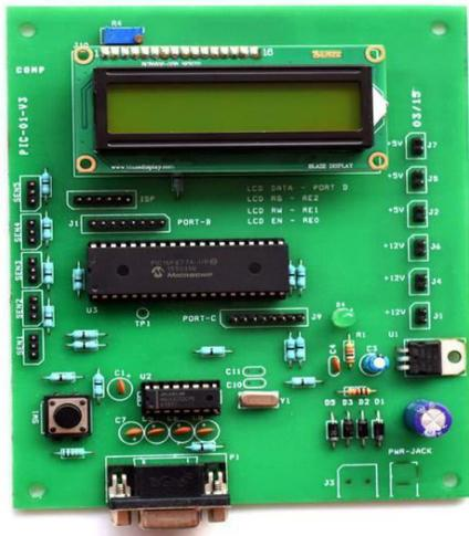
FIG 6: PIC ASSEMBLED PCB+UART+LCD
