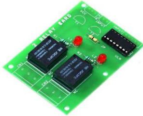
Fig 5: Two Relay board
