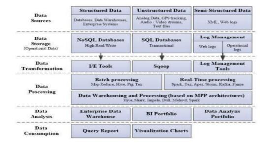
Figure: 4 the architecture of a BD integration ecosystem
