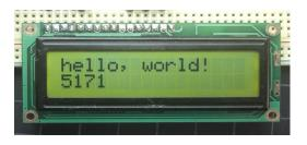
Fig -6: Liquid Crystal Display
