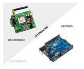
Fig -4: GSM Module
