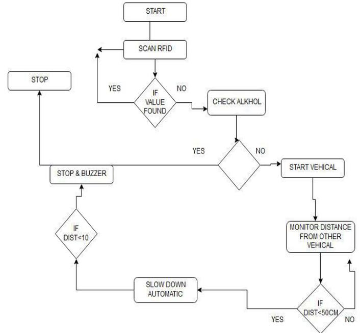
Fig. Flowchart of Accident Prevention System
