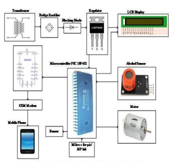
Fig. Architecture of the System
