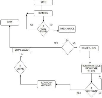
Fig. Flowchart of Accident Prevention System
