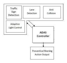
Figure 2. proposed system architectural block diagram
