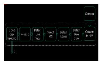
Figure 7. The Lane Detection Process
