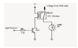
Fig -4: Relay Driver Circuit
