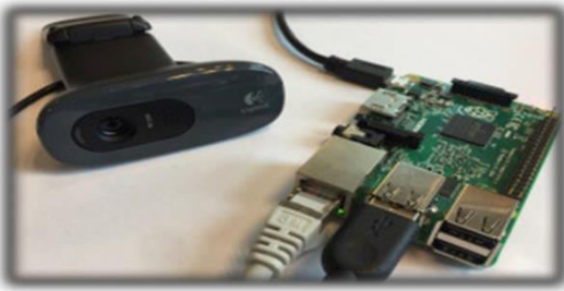
Fig. 7 Integration of components with Raspberry Pi
