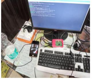
Figure 7. Result of wirelessly camera module to show vehicle front view in mobile display
