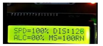
Figure 8. Result of speed, distance, alcohol and Rf signal is showing in LCD display
