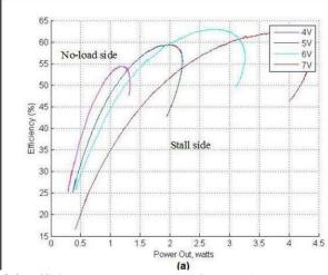
Fig3.2 Efficiency vs. power output for BLDC motor (100% throttle and varying voltage).
