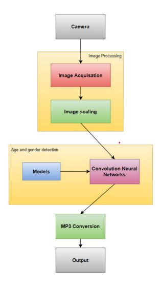
Initially, from the camera the video is captured and then converted into frames. Once the we get a frame from the live video stream, image acquisation process is done. Then image scaling is done to the required dimensions and then finnaly fed as the input to the three layer convNet layers. There the age and gender are classified with the help of the age-caffe model and gender-caffe model.
