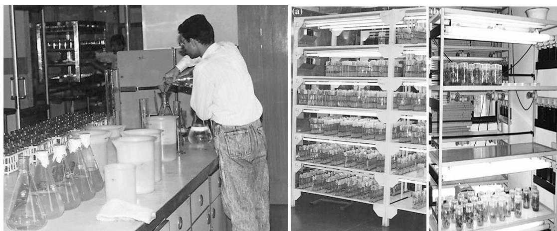
Fig3.13(f) An illuminated culture trolley with six shelves holding culture tubes arranged in metallic racks. An enlarged portion of a trolley with cultures in screw cap bottles. (Source-Bureau of Indian standards)
