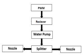
Fig-10: Block Diagram of Spraying Mechanism
