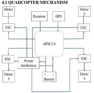
Fig-9: Block Diagram of Quadcopter
